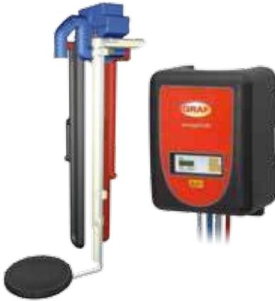
The system pack Klaro E Professional (▶ page 8) works according to the SBR air lift pump process. This requires a sewage reservoir with two chambers. Scope of supply: switch cabinet with air compressor for internal mounting, system pack Klaro E Professional comprises air lift pumps and plate ventilator. Air hose not included.
