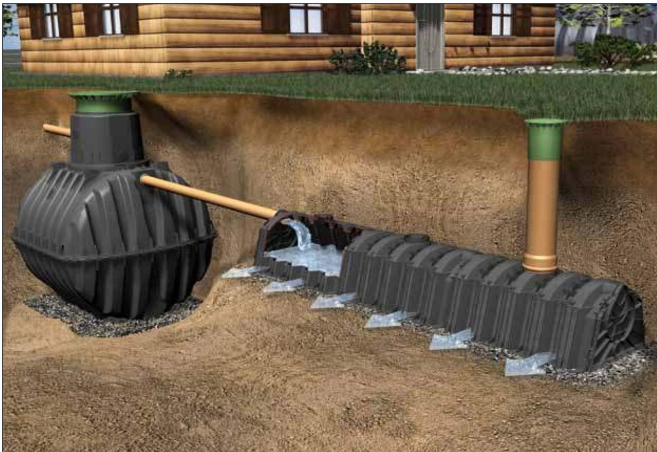
The Graf Infiltration Tunnel has been mainly designed for the use in private and rural areas. The system which consists of one or several tunnel modules and two end plates can be extended at will. The laying is realized in one or more lines of the same level. As the weight of one module is only 11 kilos, the handling of the Infiltration Tunnel is excellent.
